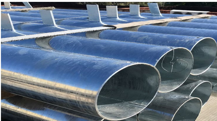
Hot Dip Galvanised is a much cleaner finish
